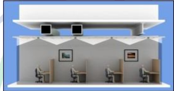
Figure 2. Ultra-wide dispersion emitters radiating directly into the listening space below results in spatial variability of less than 1 decibel throughout the office.
